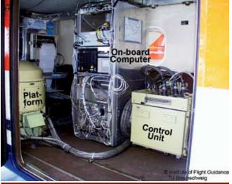
FIGURE 8 Gravity measurement system in the test aircraft
